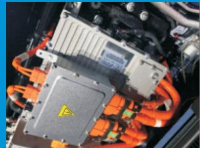
Electric vehicle high voltage wire harness is mainly used to connect the high voltage equipment of electric vehicle, such as the connection between battery pack and multi-in-one, the connection between AC charging socket and OBC, and so on. It involves the requirements of reliability, safety and other aspects, and is the key part of electric vehicle.
